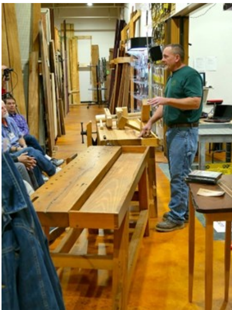
Will discusses the various features of the Moravian workbench, including the tool tray, splayed legs and the leg vise (photos: Mark Firley)
