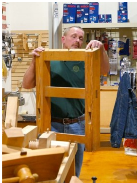
Will discusses the various features of the Moravian workbench, including the tool tray, splayed legs and the leg vise (photos: Mark Firley)
